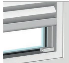
Mounting in the glazing bead with footplates.
