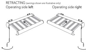
Rotate the crank clockwise - Awning retracts - Rotate the crank anticlockwise - Awning retracts -
