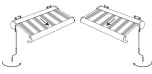
Rotate the crank anticlockwise - Awning extends - Rotate the crank clockwise - Awning extends -
