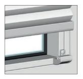
If it is not possible to mount in the glazing bead, e.g. if the glazing bead is very narrow, the glazing bead support can also be used for front installation mounting or an angle bracket (not shown) can be used on the window frame
